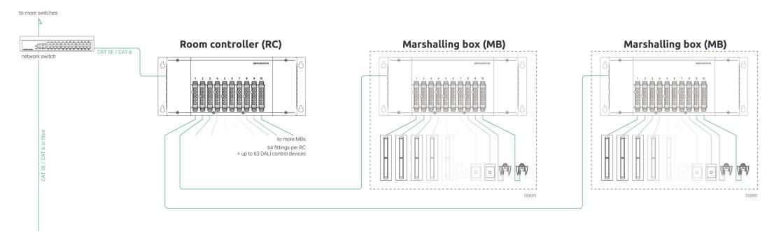
1 x RC = 64 luminaires(ECG), 63 DALI devices(ECD)
