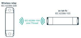
2 104 + 101 Bridge mode is enabled after the device has been added to a 104 controller and a 101 power supply has been connected to the DALI terminals.
