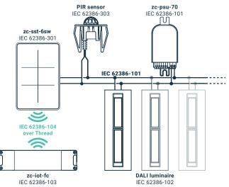
101 mode is enabled after a 101 power supply has been 3 connected to the DALI terminal and the device has not been added to a 104 application controller.
