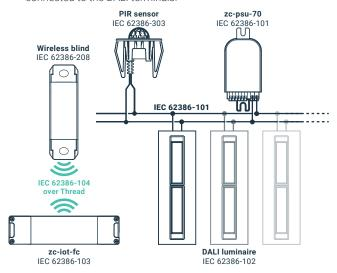
3 **101 mode** is enabled after a 101 power supply has been connected to the DALI terminal and the device **has not** been added to a 104 application controller.
