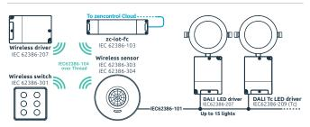
**Note** The zc-pms-iot-2sw-r or zc-pms-iot-2sw-vf smart sensor supplies 35 mA of DALI current and does not require external DALI power supply. When used with zc-iot-fc the device will act as a bridge between IEC62386-104 to IEC62386-101.
