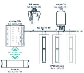
**101 mode** is enabled after a 101 power supply has been connected to the DALI terminal and the device **has not** been added to a 104 application controller.
